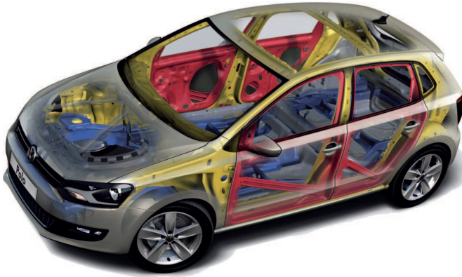
Figure 1.1 Car body structure of a Volkswagen Polo [149]
