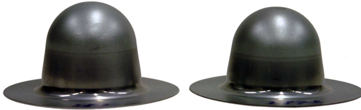
Figure 8.9 Side view of successful products obtained in the deterministic optimum (left, h = 69 mm) and robust optimum (right, h = 65 mm)
